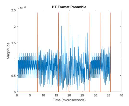
Demodulate the L-LTF and estimate the channel.
